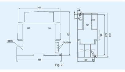
□ Geometric installation dimension of 30~37KW
